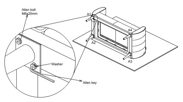
Fix part-A and Part-B by allen bolt M8x20mm and washer using Allen key at position A1,A2,A3&A4 as shown in Fig
